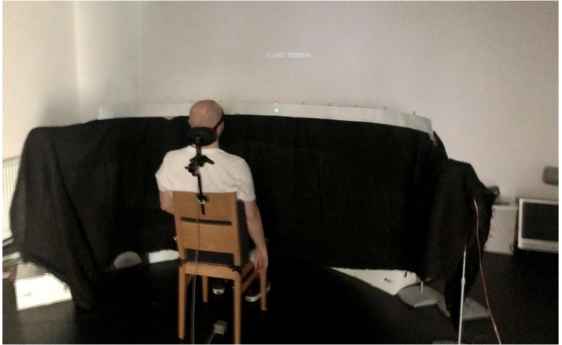
Figure 2: Room for RE part of the experiment. Chair in the middle of a semicircle of loudspeakers covered with black cloth and with a stripe of paper on top of them for presenting visual stimuli.
